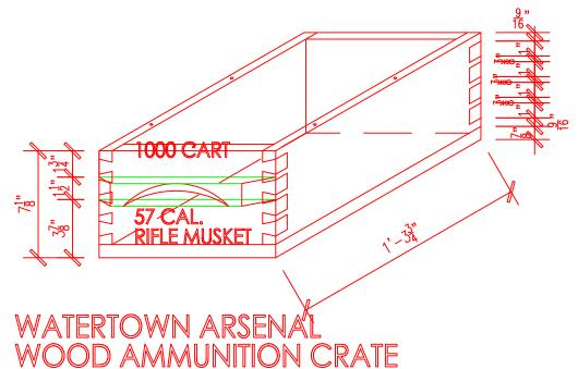
BOX IS CONSTRUCTED OF 7/8" THICKNESS BOARDS
