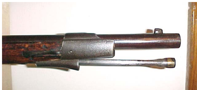
Nose cap and front barrel band, also showing the peculiar brass-sleeved rammer (all photos by John Tobey)
